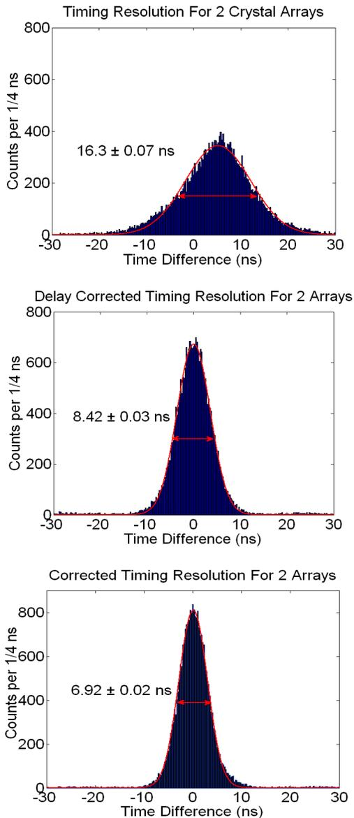
Fig. 8. Timing histograms of coincidence timing between arrays. From top to bottom: No correction, FWHM 16.38±0.05 ns; ASIC inter-channel delay correction, FWHM 8.42±0.03 ns; and inter-channel delay, signal amplitude and quadrature timing correction, FWHM 6.92±0.02 ns.
