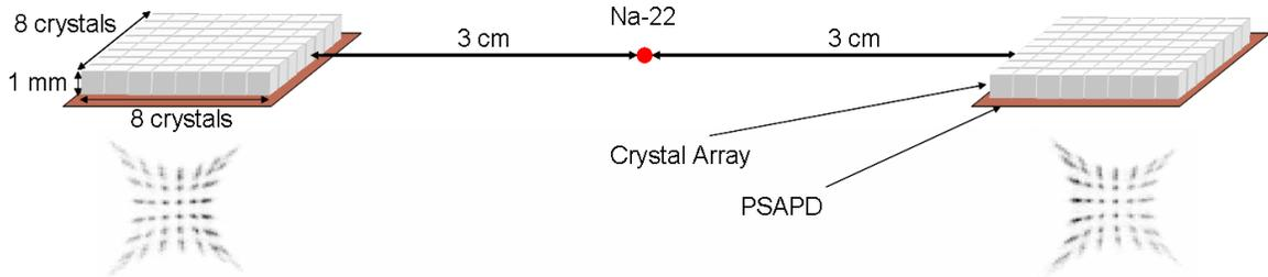
Fig. 7. Two 8x8 1x1x1 mm<sup>3</sup> crystal arrays coupled to PSAPDs are placed edge-on, 6 cm apart. A <sup>22</sup>Na point source is placed in between the two crystal arrays. The crystal flood histogram for each array used for crystal gating is shown below the crystal.
