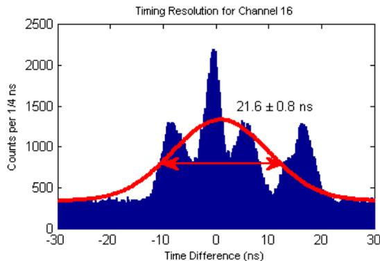
Fig. 3. The pulser timing histogram is shown from one channel to 10 other channels. Randoms are added to the data set and are visible as the constant background level in the histogram. The individual channel delays are visible as the several peaks in the figure.
