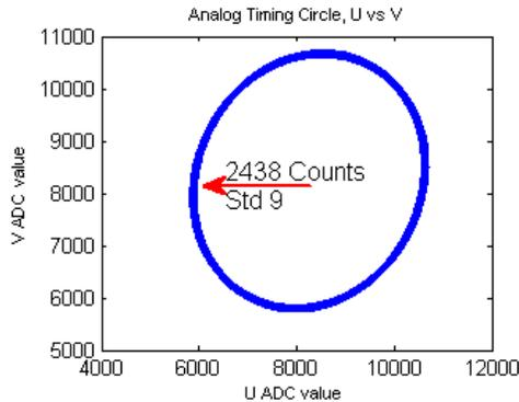
Fig. 2. The quadrature timing signals, U and V, when plotted against each other for many events, form a circle. The fast timestamp is determined by the angular separation of the two events on the circle.
