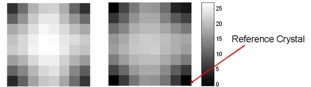
Fig. 9. The optimum delay adjustment for the two 8x8 crystal arrays. The color scale is in nanoseconds.
