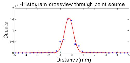
Fig. 10. Histograms of the lines of response from the coincidence data with a 0.250 mm diameter point source with a 0.33 mm pixel/bin size. The bottom plot is a histogram of the lines of response taken from a vertical profile through the center of the point source. The raw FWHM is 0.90 ± 0.05 mm (before beam size deconvolution).
