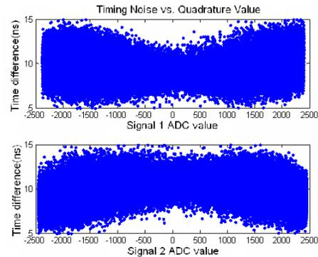
Fig. 4. Plotting the quadrature timing signals against the calculated time difference shows a strong correlation which can be corrected to improve the timing resolution.
