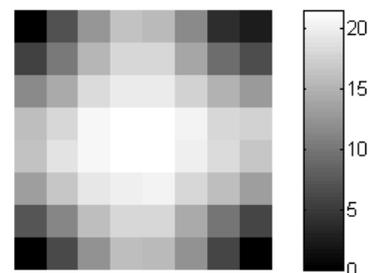
Fig. 5. This color map shows the per crystal timing delay caused by the PSAPD resistive sheet. The color scale units are nanoseconds. The bottom right corner is the reference timing.
