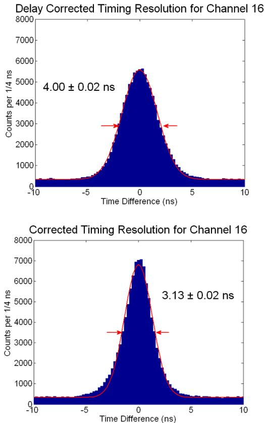
Fig. 6. Timing histograms from one ASIC channel to the other 10 channels using pulser data. Top, the FWHM improved from the uncorrected  $21.6 \pm 0.8$  ns to  $4.00 \pm 0.02$  ns after ASIC inter-channel delay correction. Bottom, correction for quadrature timing correlated noise gains another 22% improvement to achieve  $3.13 \pm 0.02$  ns.
