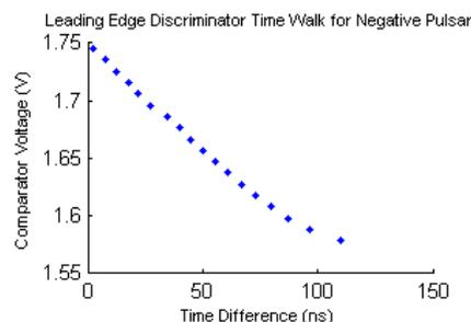
Fig. 1. Changing the threshold value on the leading edge discriminator trigger shows the shape of a pulser. Lowering the threshold causes the negative pulse to fire the comparator at a later time.
